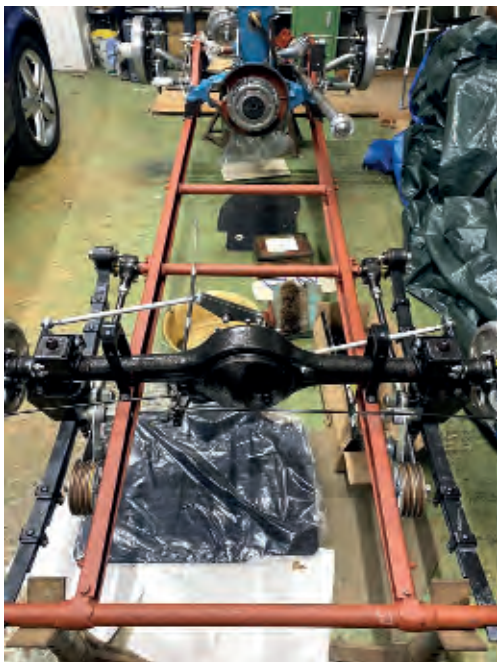
EX149: Progress photos – Chassis and rear axle.
