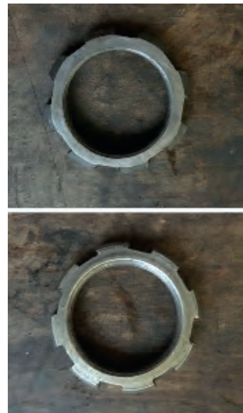
The slots in the new slotted nut (bottom) are much deeper than in an original style nut (above) which reduces the bearing surface area and potentially weakens the nut
